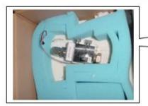
NOT packaged correctly – loose allowing cell movement and potential damage during transport
